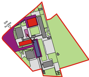
Phase 4 Decant block 2 to temporary accommodation Remodel block 2 including new lift (4 storey)
