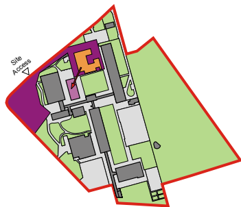
Phase 1 Decant block 3 to temporary acc. (24 general teaching and 4 specialist teaching rooms during duration of construction programme) Demolish block 3
