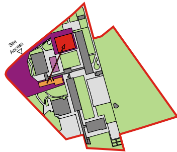
Phase 2 Build new Entrance / Admin. / 6th form / General Teaching block and new skills centre (2100 m 2 - 3 storey) Decant block 5 Entrance / Admin. / 6th form to new block Demolish block 5
